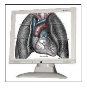
17 inch LCD with a 4:3 aspect ratio. This unit is water sealed with an anti-glare glass front. Capable of 16.7 million colors and a resolution of 1280 x 1024. The 17 inch monitor has a viewing angle of 170 degrees and a response time of 15/10 ms. This unit is cart or wall mountable and has video inputs for VGA, Composite or S-Video. The monitor is compatible with NTSC, PAL or SECAM.
