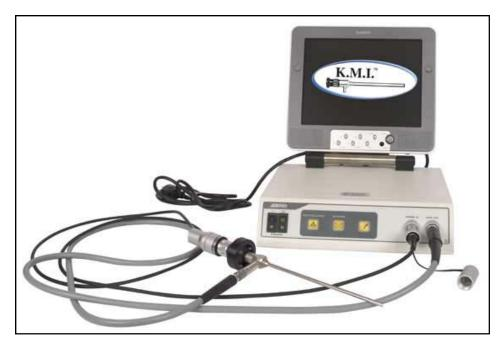
This system is a combination of a high intensity Xenon light source, USB port for digit photo capture and download, a color CCD camera system, endoscope coupler, fiber-optic lighting cables and a 12 inch color LCD all enclosed in a compact portable design. The camera features an automatic shutter, single chip and is soakable. The Camera Combo Unit is universal voltage compatible for use anywhere in the world.
